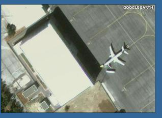
Aircraft Hangar (5,641 sqm) **Reinforced Concrete, Steel Roof** 24 m Height **Ground Floor Administrative Sections Rest Rooms, WC & Showers Warehouse and Workshops Electrical and UPS Room Filter Washing Room Security, Heating Room**
